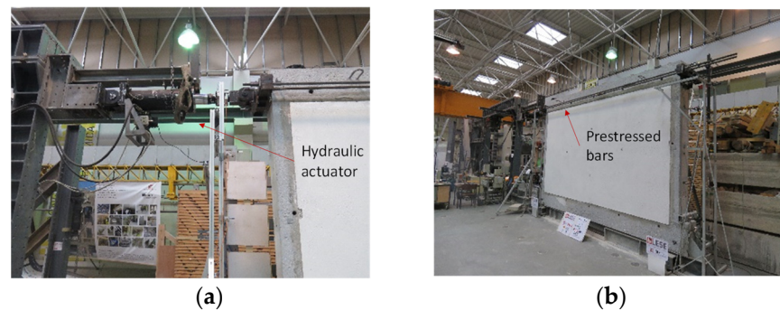
Figure 3. Test setup of the in-plane experimental tests: (a) detail of the hydraulic actuator; and (b) lateral view.
