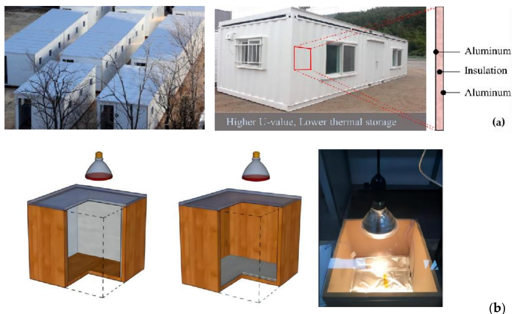
Figure 1. (a) Temporary hospital units in Seoul Medical Centre, Korea. (b) Schematic diagrams of box experiments on the thermal properties of PCMs. Reprinted with permission from Ref. [6] ©2021, Elsevier Ltd.
