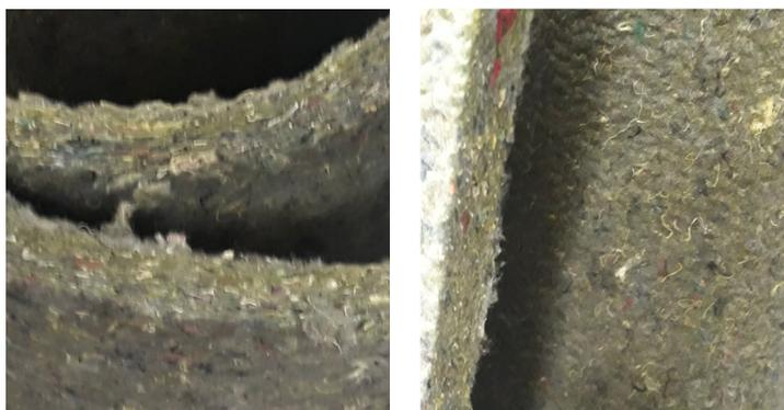
**Figure 2.** Materials: the textile felt (FLT).
