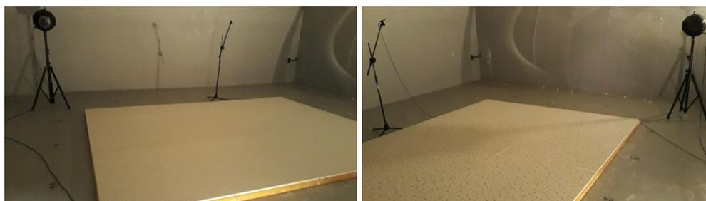
**Figure 8.** Sound absorption tests in the reverberation chamber of the EPSG–UPV.
