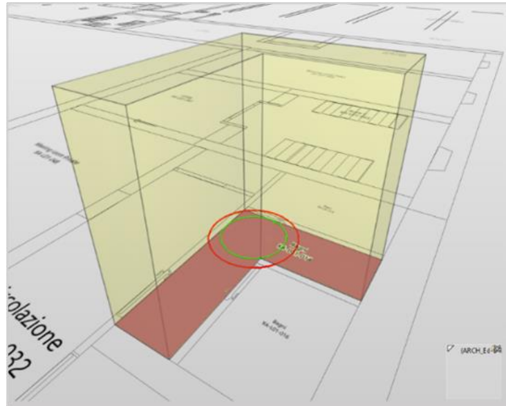
Figure 12. Results of the model check—A4 code checking. In evidence a false negative due to the intersection between the wheelchair turning circle (1500 mm diameter set within the rule) and the walls of an antebathroom.
