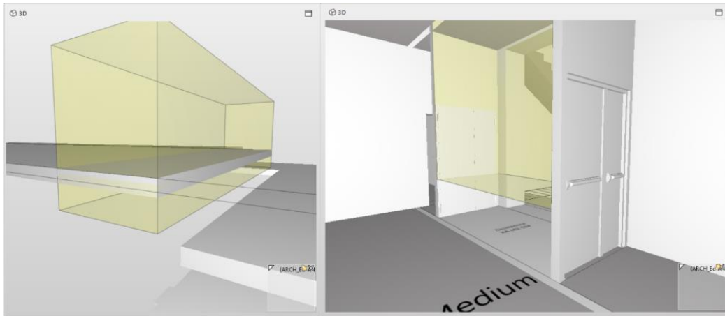
Figure 6. Environment with lower surface not in contact with any horizontal element ( left ) and environment suspended from it ( right )—C12 BIM validation.
