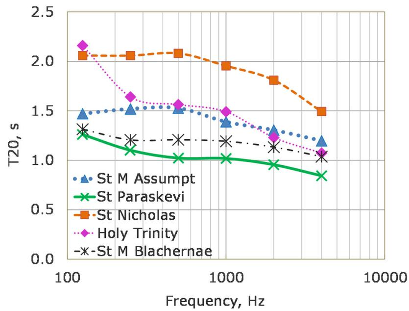
Figure 14. Measured values of reverberation time ( $T_{20}$ ).
