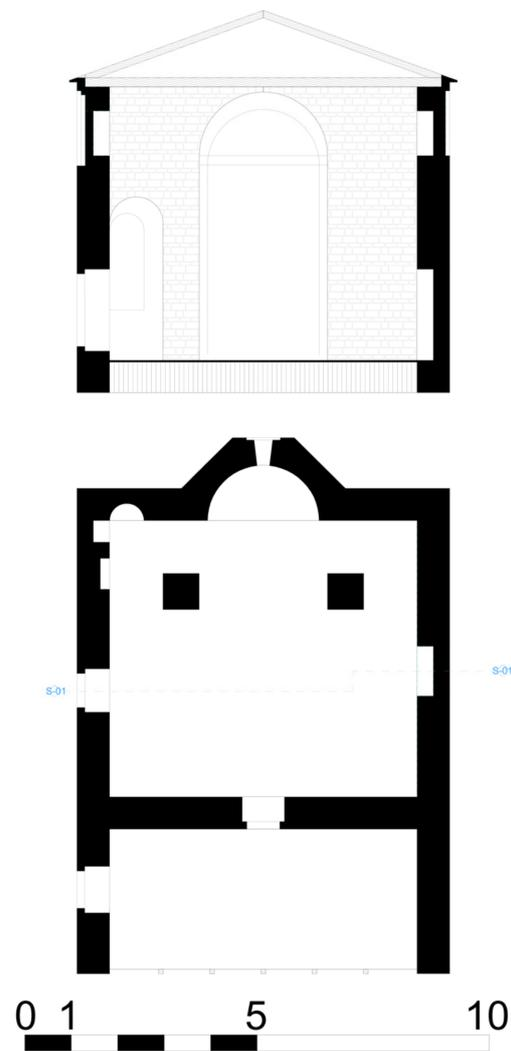
**Figure 10.** Plan layout and longitudinal section of the St Mary of Blachernae's church of Berat. Provision courtesy of Arch. Arsim Murseli, UBT University.
