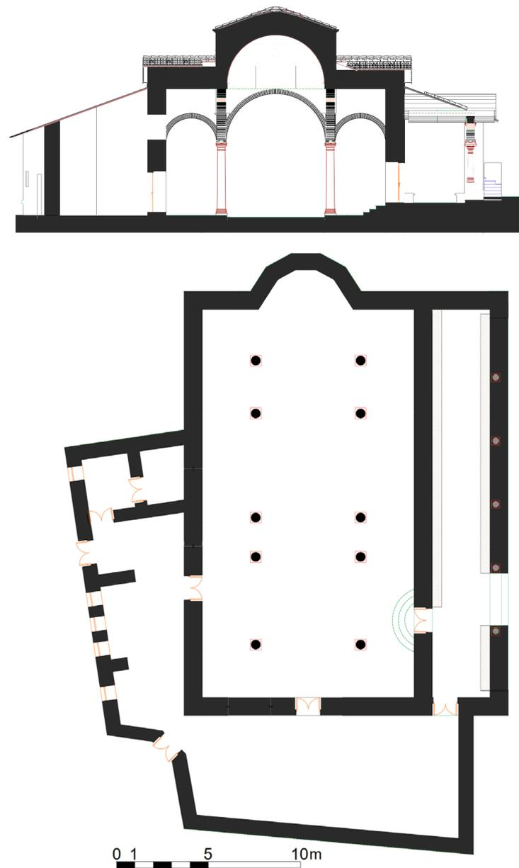
**Figure 2.** Plan layout and transversal section of St Mary Assumption's church. Provision courtesy of Arch. Arsim Murseli, UBT University, Pristina, Kosovo.
