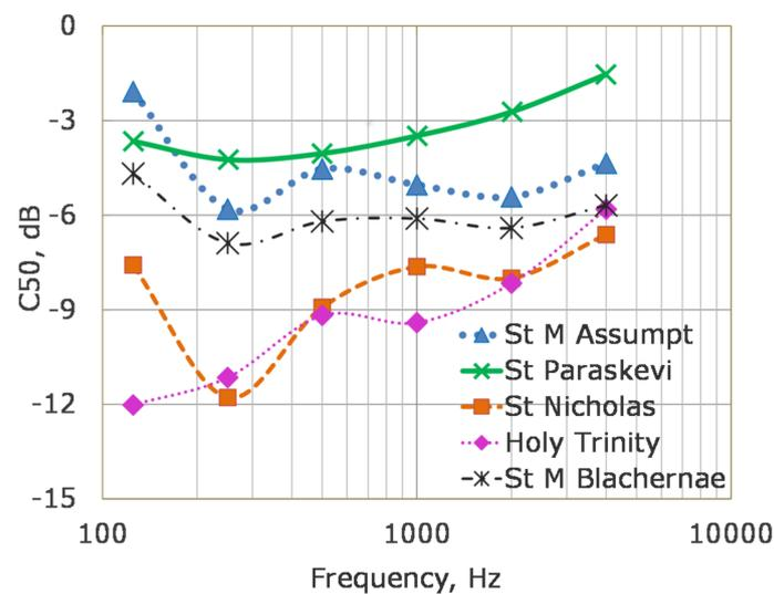
Figure 16. Measured results of clarity index ( $C_{50}$ ).
