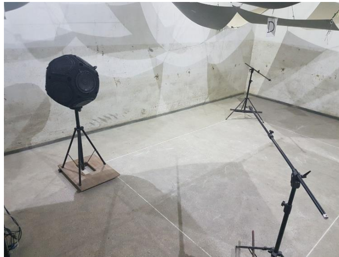
Figure 2. Microphone system—the source during the reverberation time of the reverberation room.
