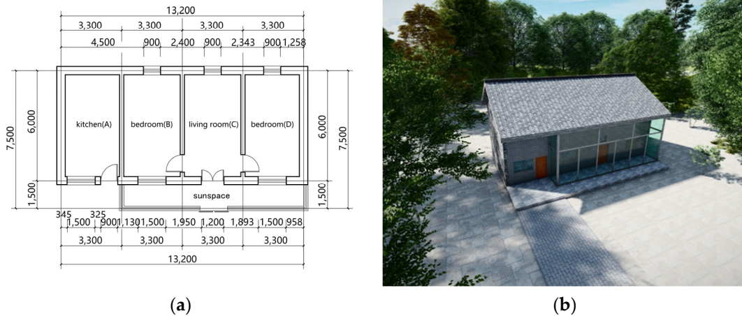
Figure 7. The improved model (a) plan of slate dwelling, (b) model of slate dwelling.
