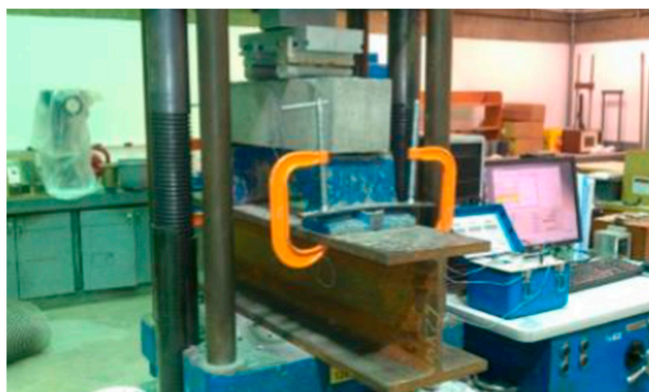
Figure 2. Detailed third-point bending test setup for a typical specimen [Reprinted/adapted with permission from Ref. [37]. 2022, Elsevier].
