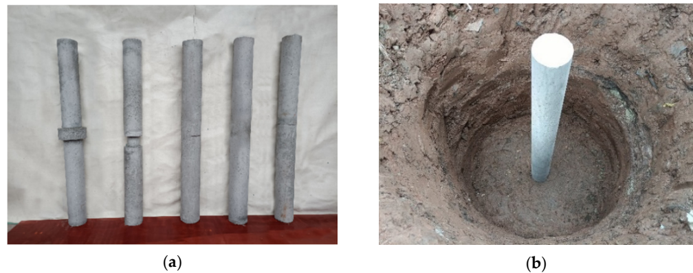
Figure 8. (a) Experimental piles (bulge imperfection; neck defect; crack; weak concrete; broken); (b) Placement of experimental pile.
