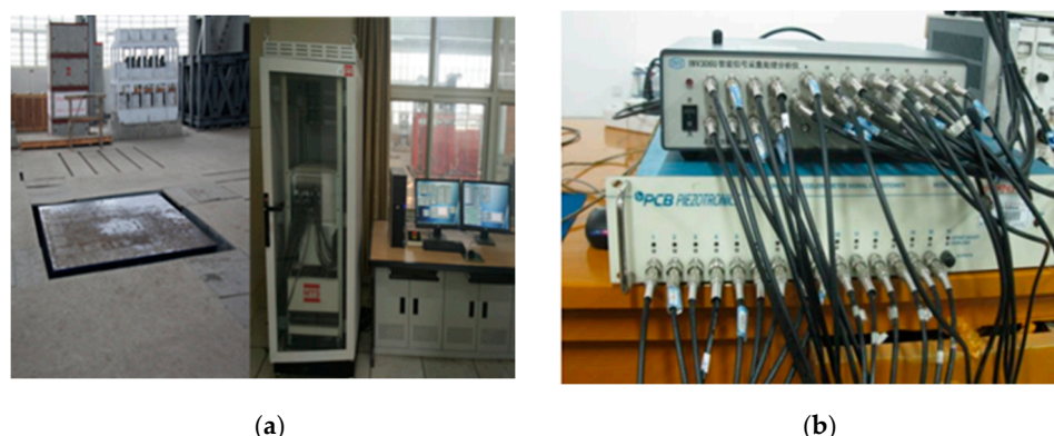
Figure 5. Testing equipment. (a) Field of shaking table and control system; (b) LMS data acquisition instrument (under test).
