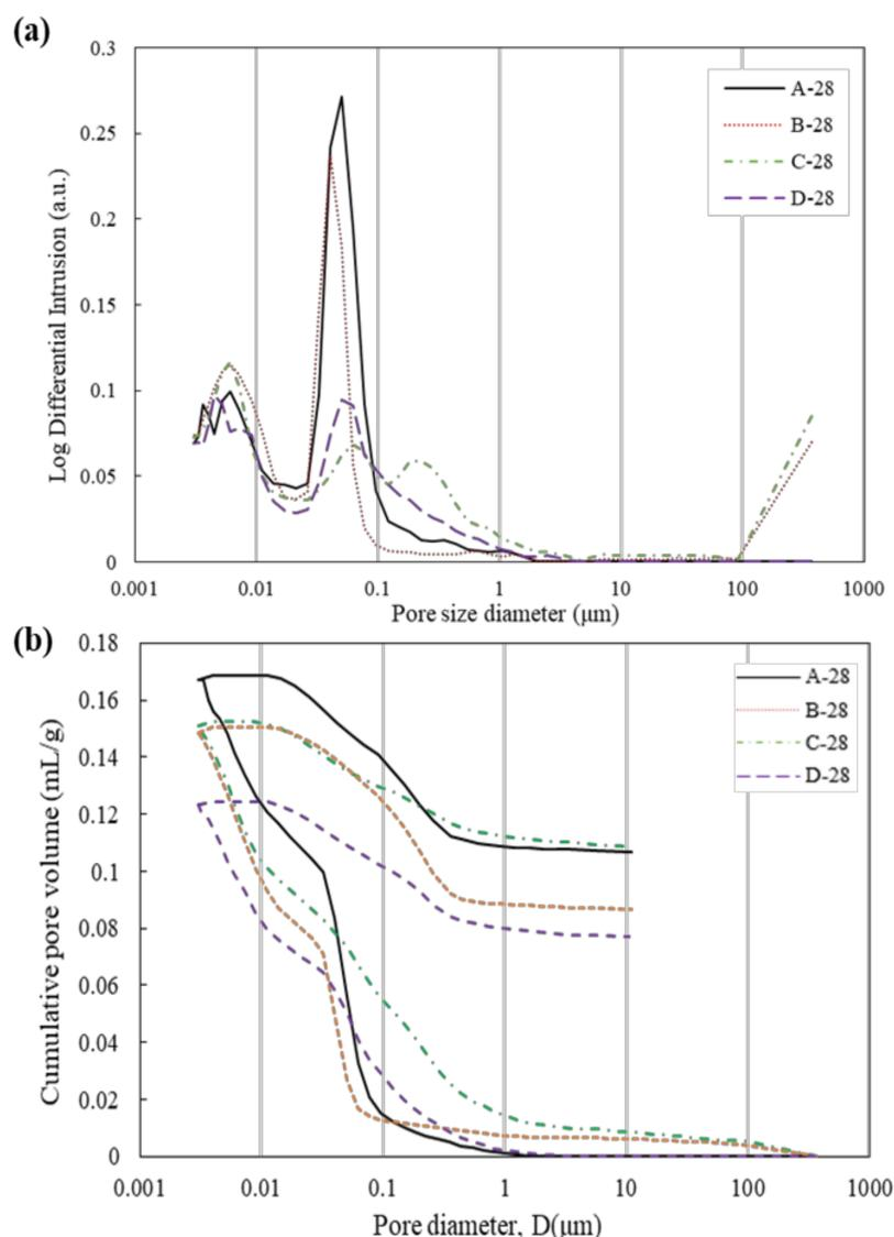
**Figure 4.** (a) Log differential and (b) cumulative intrusion/extrusion curve by pore size diameter of paste specimens after 28 days of curing.
