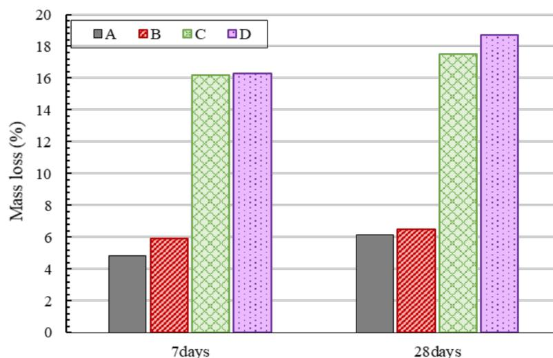
**Figure 7.** Mass loss (%) of  $\text{CaCO}_3$  calculated from TG curves in paste specimens after 7 and 28 days of curing.
