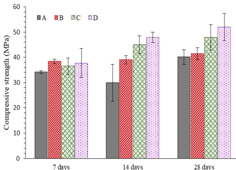
**Figure 3.** Compressive strength values of paste specimens after 7, 14, and 28 days of curing (A and B specimens: without and with bacterial culture solution in water curing, respectively. C and D specimens: without and with bacterial culture solution in carbonation condition, respectively).
