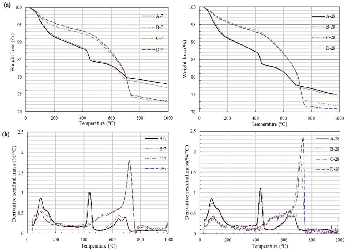
Figure 6. (a) Thermogravimetry (TG) and (b) Differential thermogravimetry (DTG) analysis results after 7 and 28 days.
