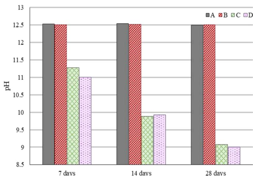
**Figure 8.** pH evolution of paste specimens after 7, 14, and 28 days of curing.
