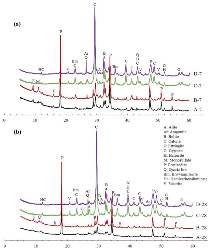
Figure 5. X-ray diffractometer (XRD) analysis of paste specimens after (a) 7 and (b) 28 days.
