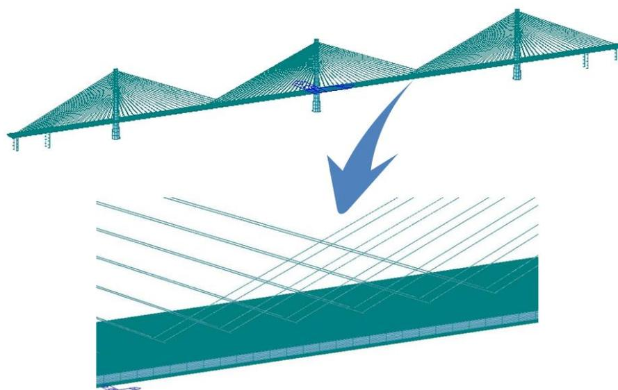
**Figure 2.** Crossed-cable model details.
