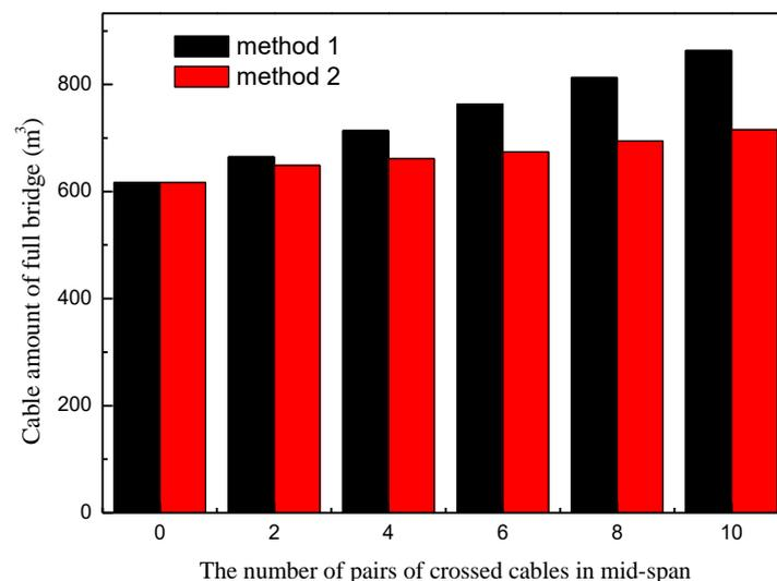
**Figure 10.** Comparison of the consumption of the cables.
