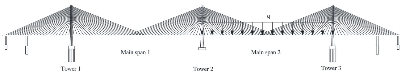
**Figure 3.** The sketch of the unbalanced load.
