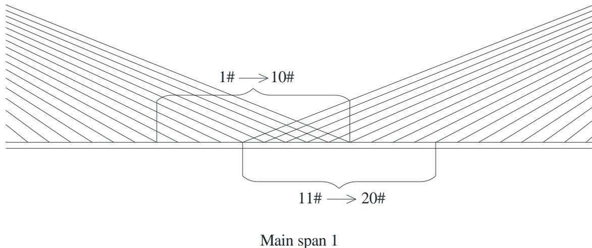
Figure 7. Numbering diagram of stay cables.
