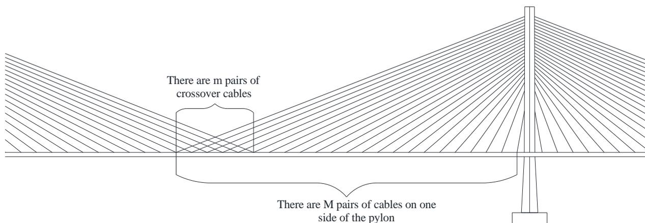
**Figure 13.** Cross-cable ratio calculation diagram.
