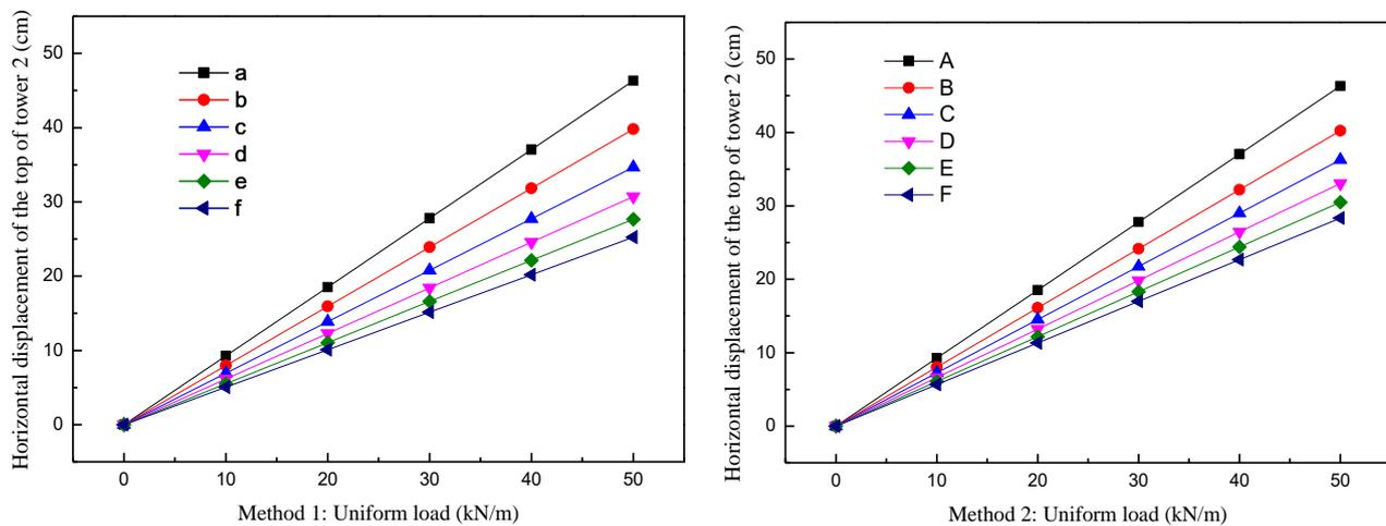
**Figure 4.** Comparison of horizontal displacement of mid-tower.
