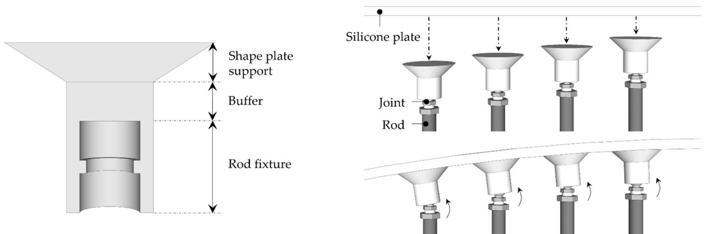
**Figure 5.** Detachable-type silicone cap.
