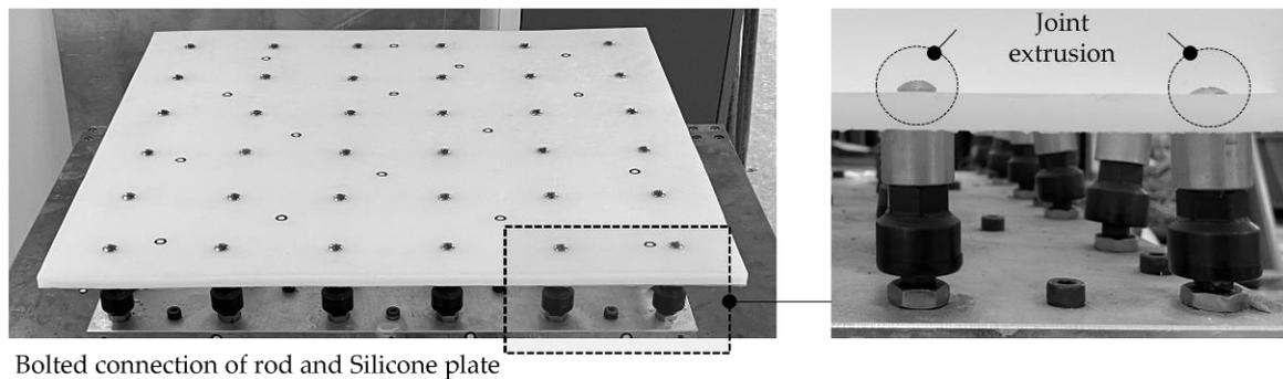
**Figure 3.** Surface of fixed-type molds.
