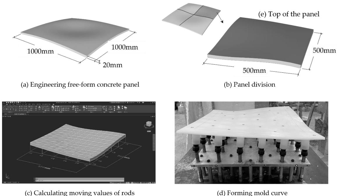
Figure 10. Shape engineering and curve forming.
