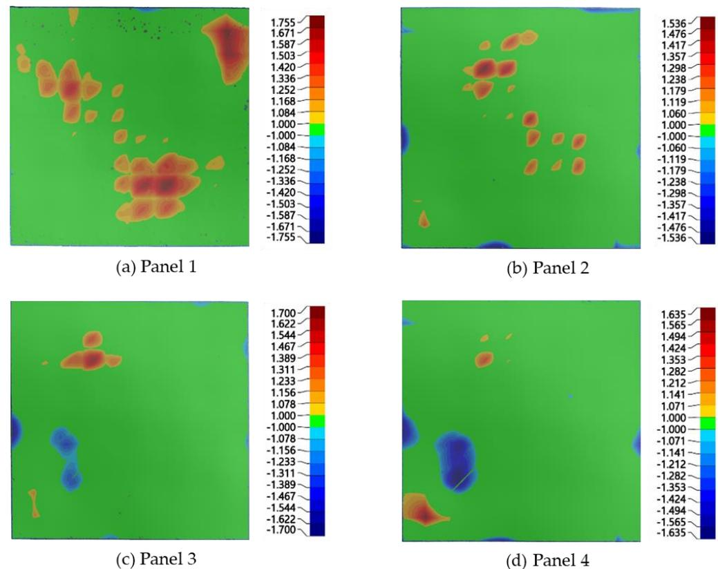
**Figure 13.** Shape error of free-form concrete panel in repeated fabrication.
