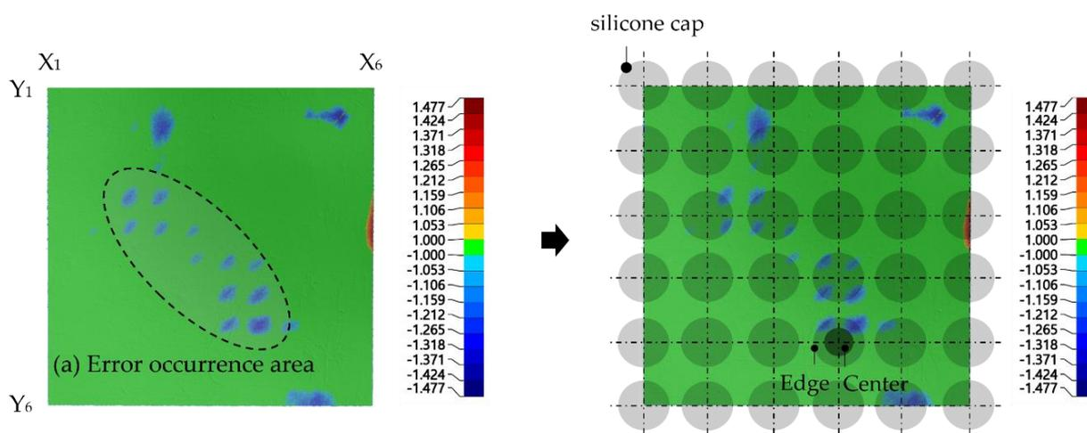
**Figure 11.** Shape error of mold curve according to the position of silicone cap.
