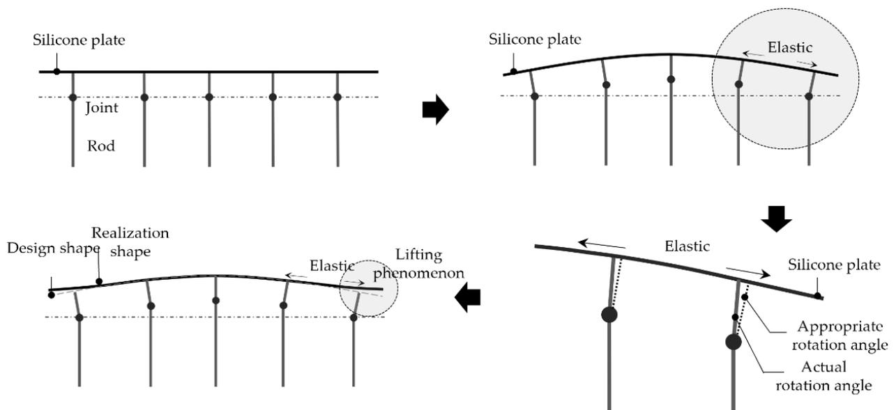
**Figure 2.** Limitation of revolving rods.
