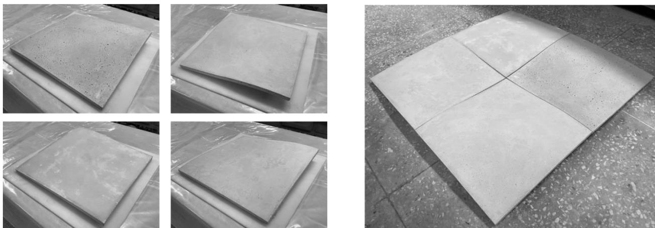
**Figure 14.** Final free-form concrete panel.
