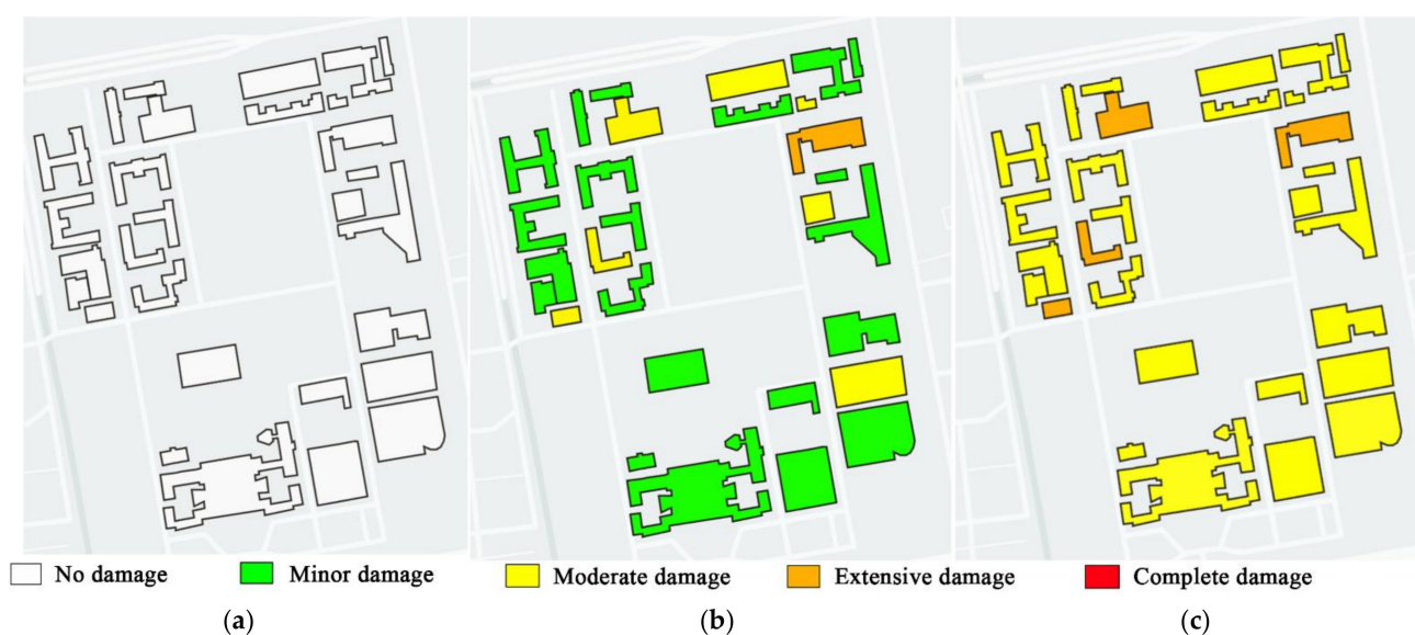
Figure 10. Structural damage states under different earthquake intensities: (a) frequent earthquake; (b) rare earthquake; (c) extremely rare earthquake.
