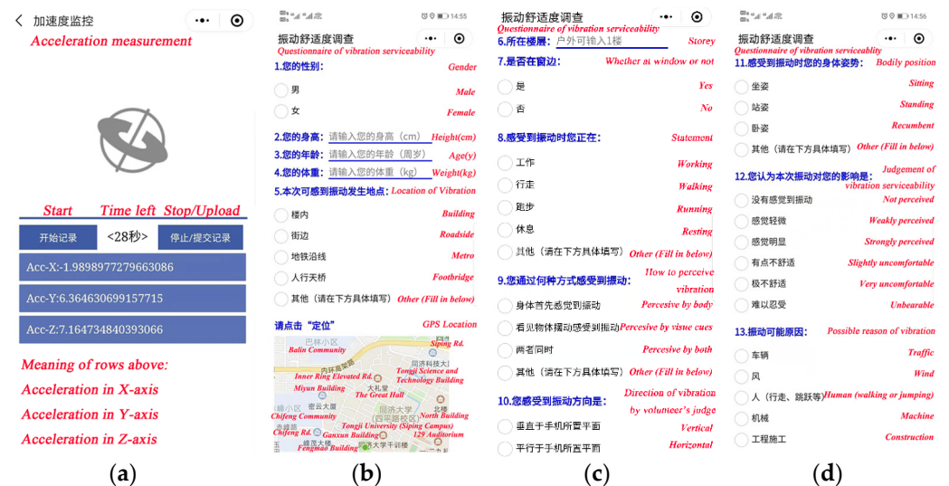
Figure 2. Vibration measurement (a) and questionnaire (b–d) in VCheck (Menu in Chinese, English translation in italic).
