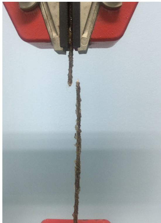
Figure 2. Test setup for the hemp rope.
