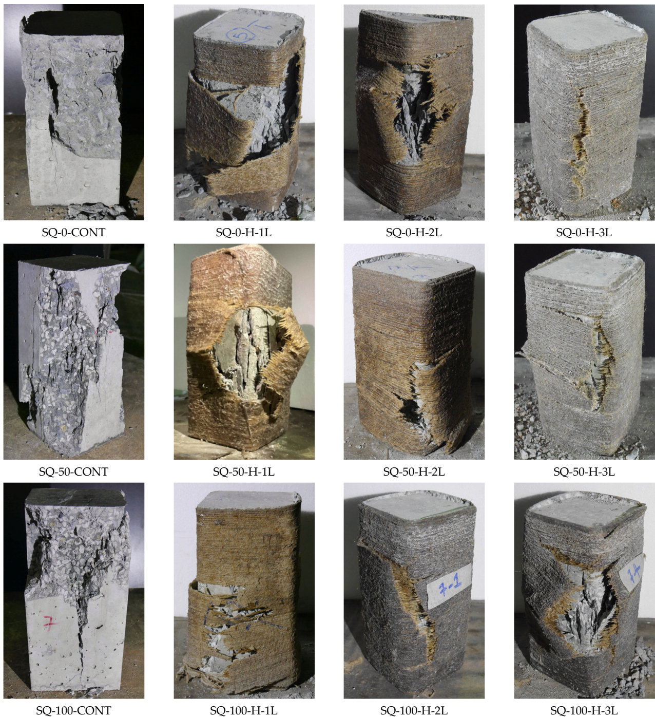
Figure 5. Ultimate failure modes of all specimens.
