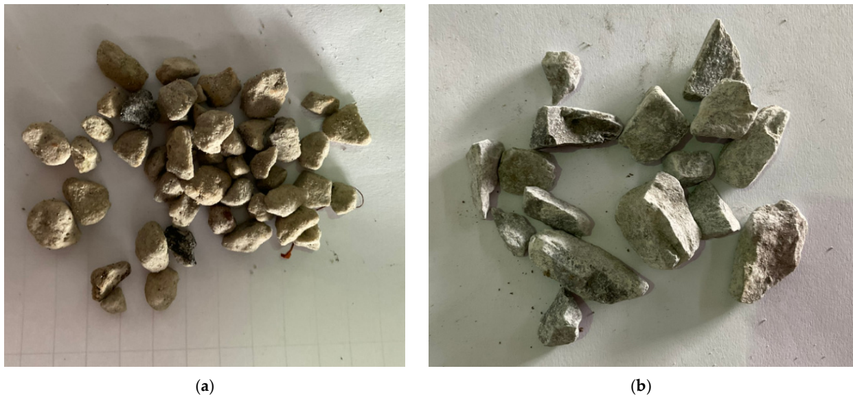
Figure 1. (a) Lightweight and (b) natural coarse aggregates.
