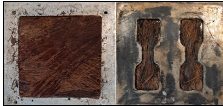
Figure 2. The two types of molds used for the DPSF/PVA composite fabrication.
