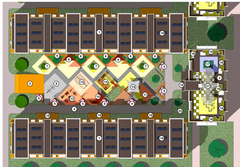
Figure 21. Residential yard reconstruction project (Author's material). 1: Reconstructed 4-story residential apartment building with an extension of an additional floor with an attic; 2: Project 9-storey apartment building with commercial premises and an operational roof; 3: Entrance to underground parking located under the yard area; 4: Fire passage; 5: Flower bench; 6: Bench with a tree; 7: Bench with apple tree; 8: Streetball sector; 9: Gazebo Type-1; 10: Gazebo Type-2; 11: Gazebo Type-3; 12: Outdoor exercise equipment sector; 13: Training horizontal bars sector; 14: Playground sector for active games; 15: Children's sandbox sector with an umbrella; 16: Flower myths; 17: Tennis tables; 18: Entrance group with a ramp under the canopy; 19: Solar panels; 20: Operated roof; 21: Decorative awnings or umbrellas; 22: Elements of landscaping.
