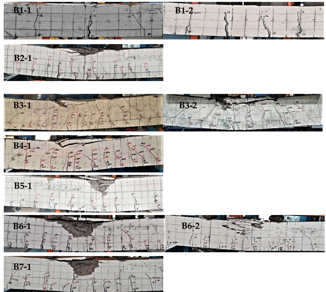
Figure 4. Failure form of test beams.
