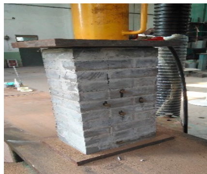
Figure 5. Compressive strength test of the masonry.
