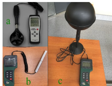
Figure 5. Test instruments: (a) Hot-wire anemometer, (b) temperature and humidity meter, (c) black globe thermometer.
