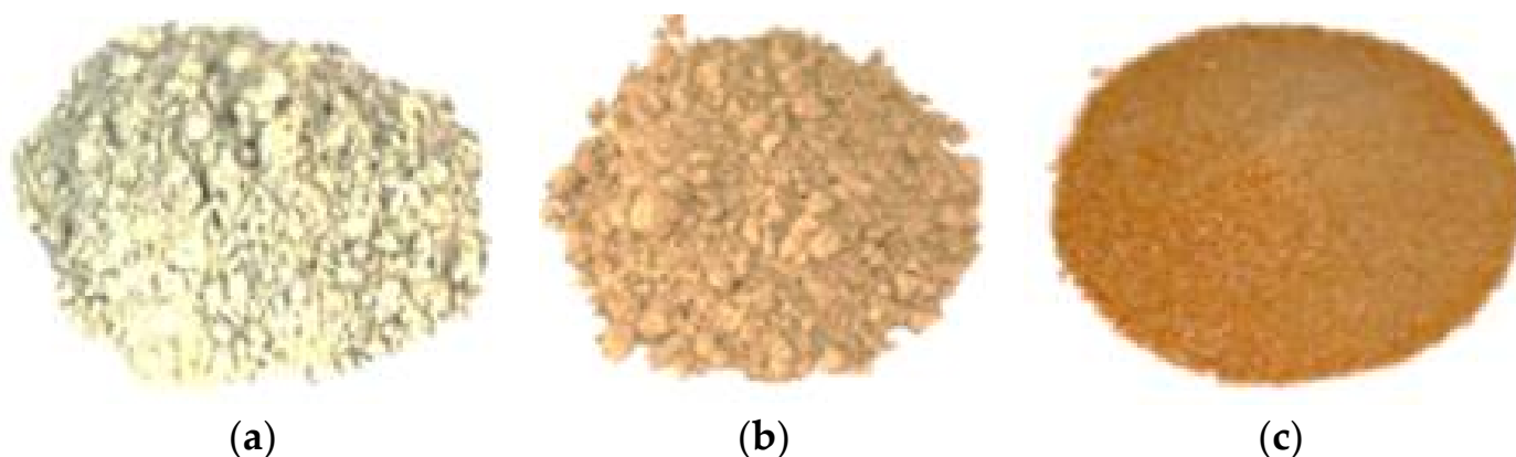
Figure 1. Physical appearance of (a) slag, (b) fly ash, and (c) dune sand.
