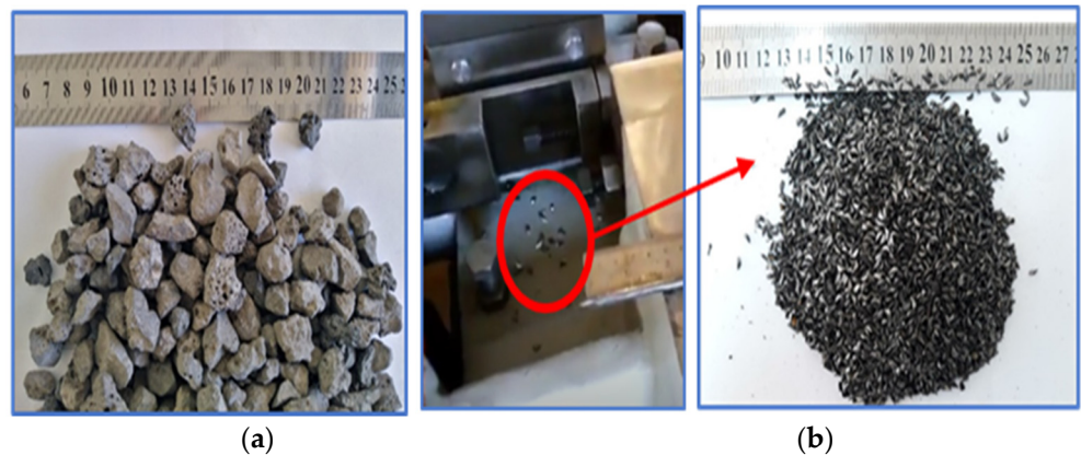
Figure 2. Particle size of fine and coarse aggregates. (a) EAFSS. (b) MNW.
