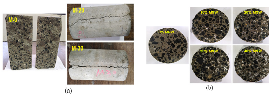
Figure 5. Effects of MNW on failure mode and distribution shape in concrete. (a) Failure mode due to tensile test. (b) Distribution shape of MNW.
