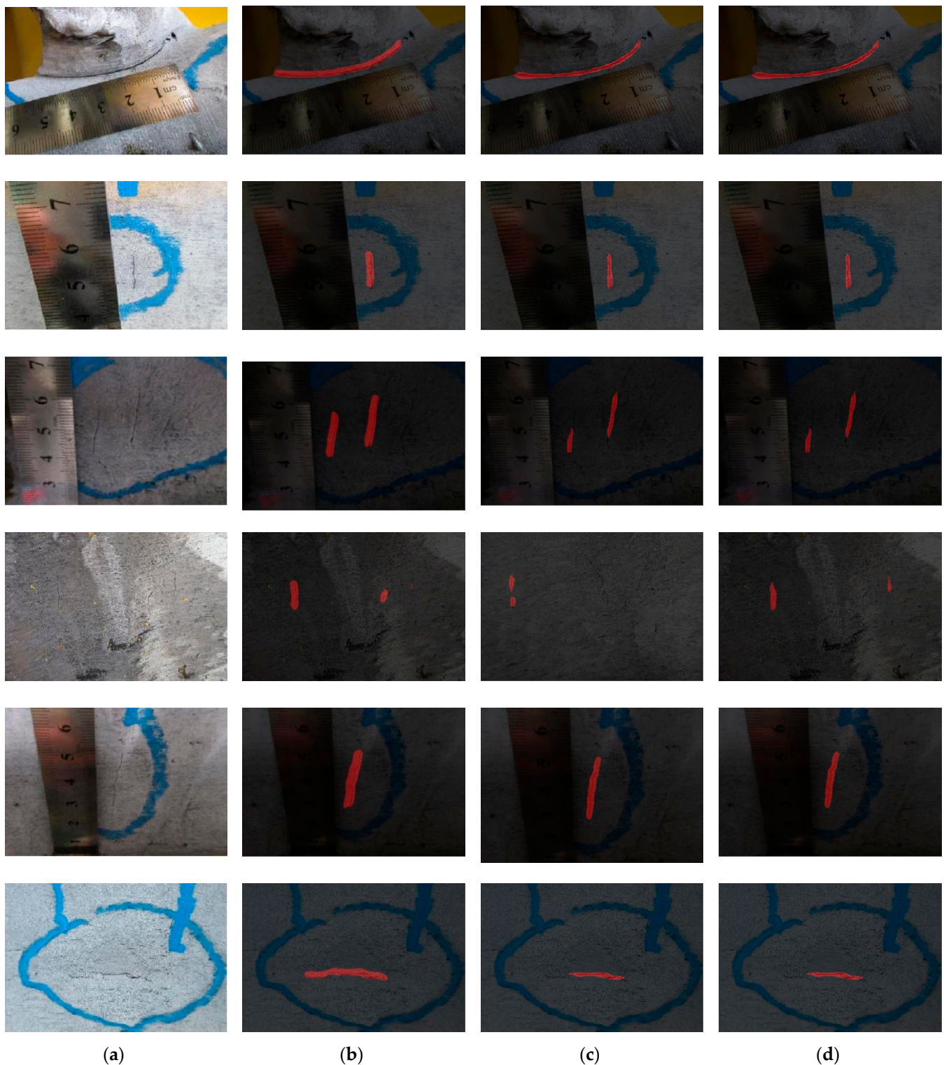
Figure 16. Results of crack identification by different semantic segmentation: (a) original image; (b) PSPNet; (c) MobileNetv2-PSPNet; (d) improved model.
