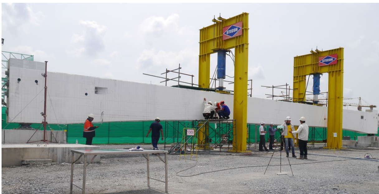
Figure 13. The two-point load applied to specimen SP-02.
