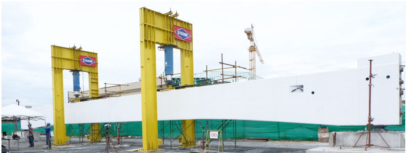
Figure 14. The two-point load applied to specimen SP-02.
