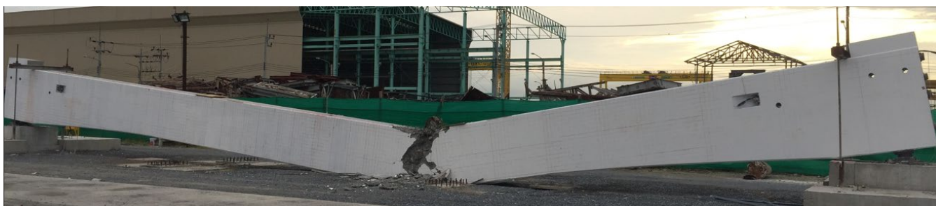
Figure 52. Ultimate failure of specimen SP-3.
