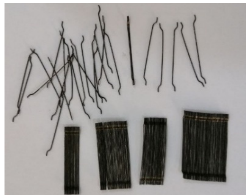
Figure 3. Used hooked-end steel fibers.
