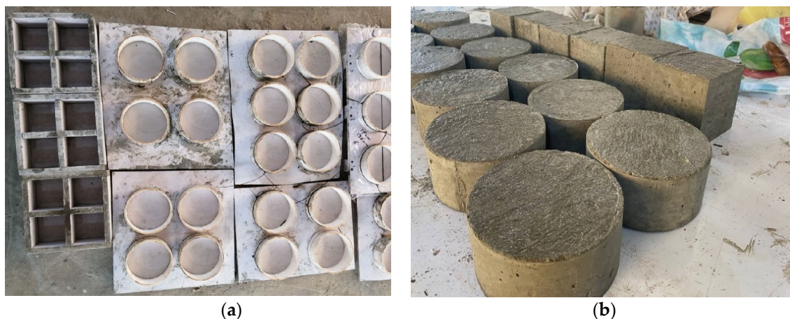
Figure 4. Impact and compressive strength specimens. (a) Specimen molds; (b) Cast specimens.
