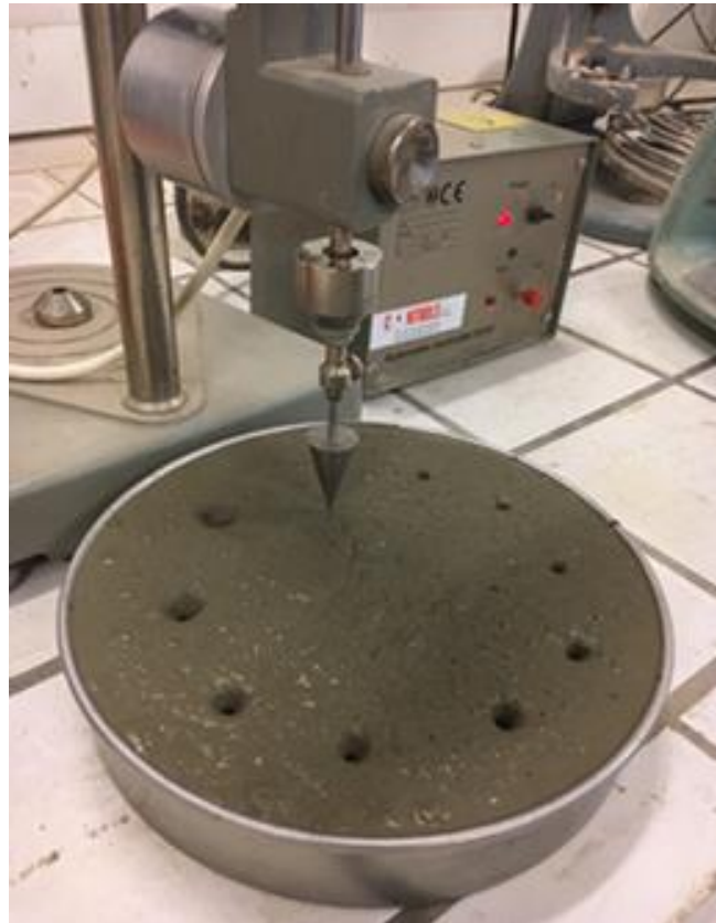
Figure 10. Fall cone test setup.
