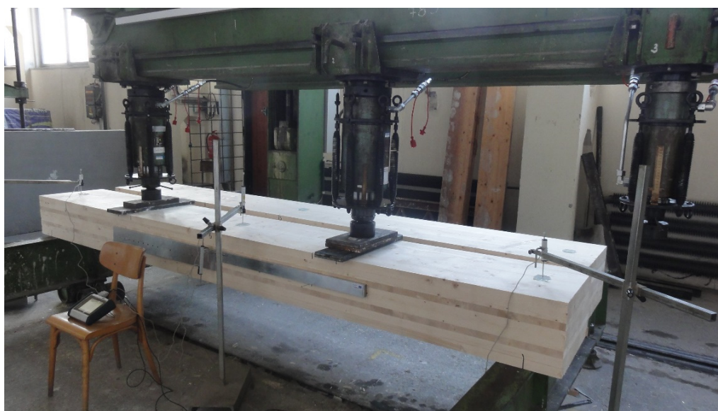
Figure 5. Test arrangement and positions of LVDTs.
