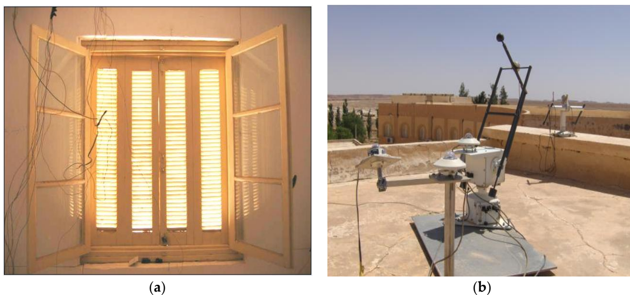
Figure 1. (a) Thermocouple position in room [15,16], (b) radiometric station in Uraer [17].
