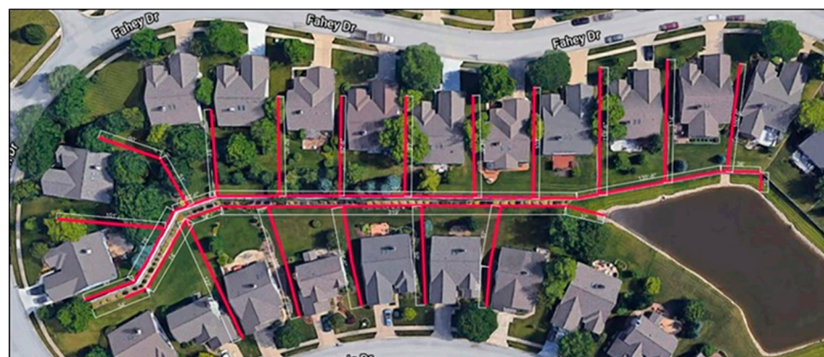
Figure A1. Drainage layout for French drain.
