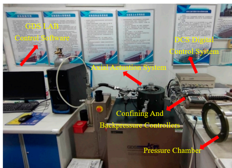
Figure 1. Dynamic triaxial testing system (DYNTTS).
