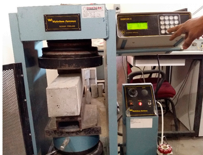
Figure 12. Modulus of rupture test as per ASTM C293.
