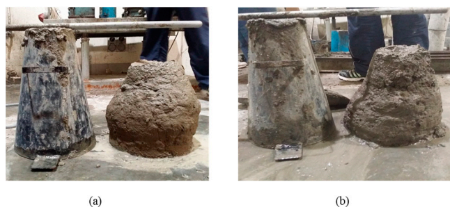
Figure 5. Slump test: (a) RA concrete (b) NA concrete.
