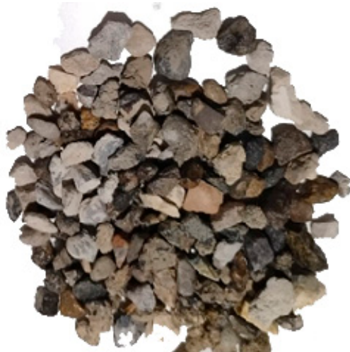
Figure 4. Sample from 20-mm-size RA.
