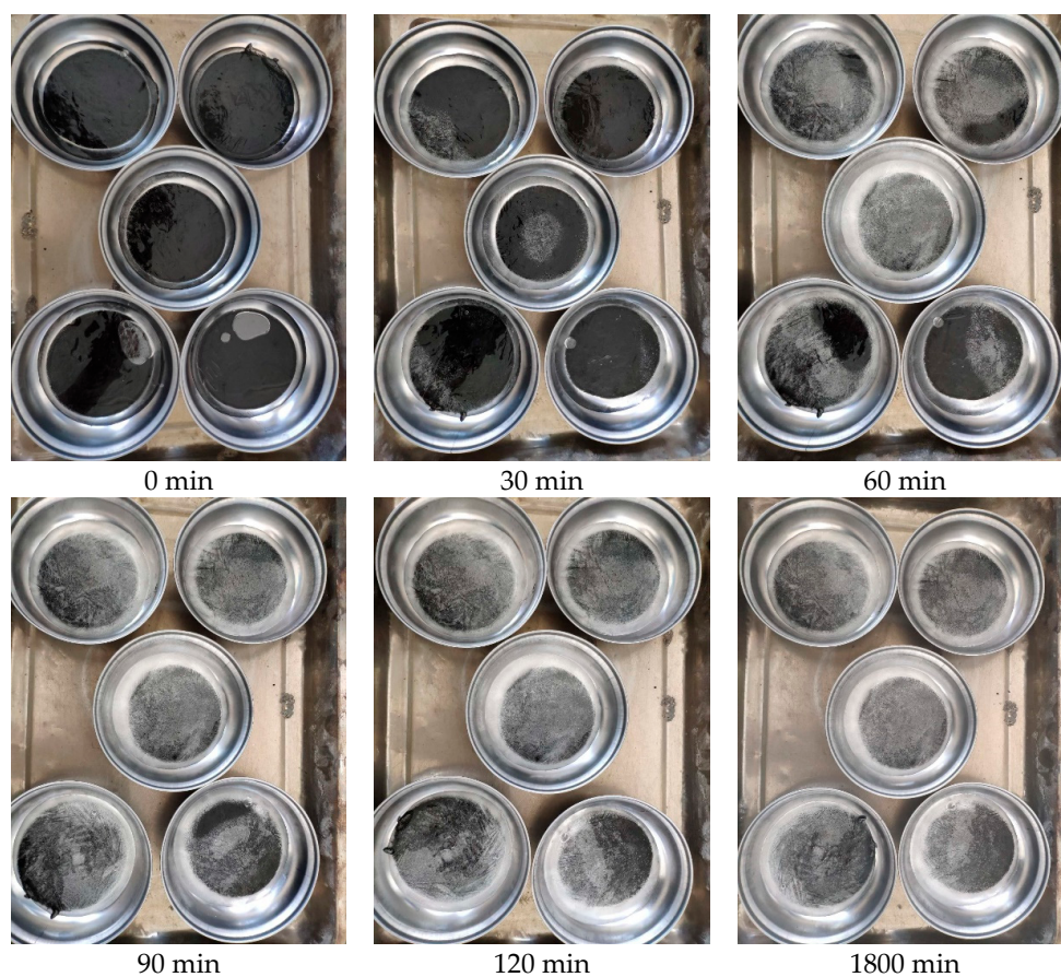
Figure 8. Freezing condition of asphalt with different contents of phase-change material at -5\text{ }^{\circ}\text{C} for different durations.
