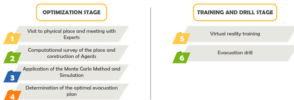
Figure 11. Comprehensive methodological proposal for modeling and simulation of evacuations in tall buildings.
