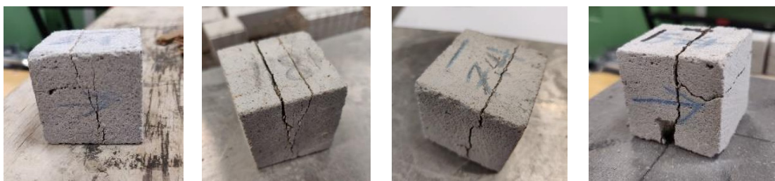
Figure 15. Fracture images of the splitting test.
