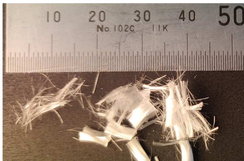
Figure 2. Polypropylene fibres, length L = 5 mm, diameter d = 0.05 mm.
