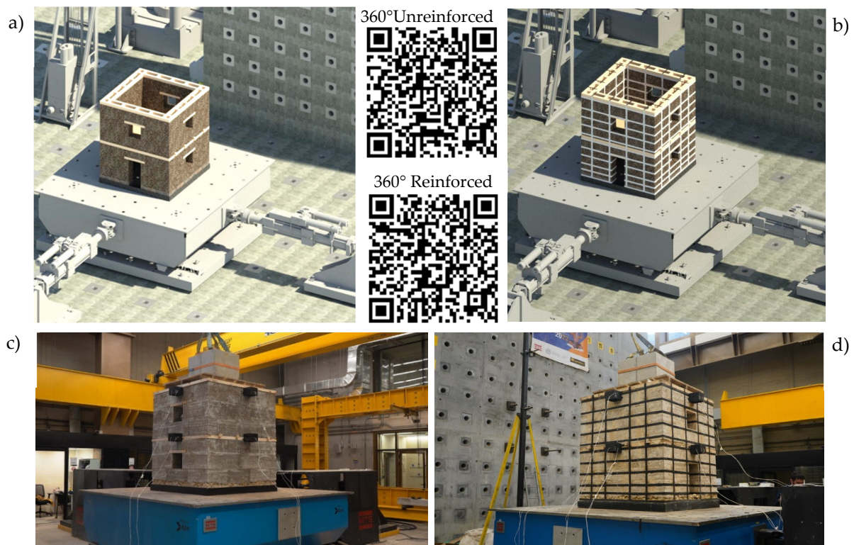
Figure 5. (a) Test set up of the unreinforced model; (b) test set up of the reinforced model. Link for QR code 360° unreinforced model: https://pano.autodesk.com/pano.html?mono=jpgs/183016e4-f29c-4ede-95c9-bfe33a7024d3&version=2 (accessed on 22 November 2023) Link for QR code 360° reinforced model: https://pano.autodesk.com/pano.html?mono=jpgs/6d32568d-f123-4ce6-9d34-4675c3ce6dc1&version=2 (accessed on 22 November 2023) (c) Photograph of the experimental setup of the unreinforced model and (d) photograph of the experimental setup of the reinforced model.
