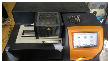
**Figure 3.** The DSC thermal analyzer.
