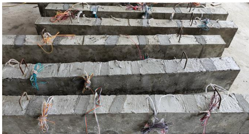
Figure 3. Maintenance of the test beam.
