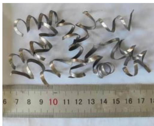
Figure 1. Recycled steel fiber.
