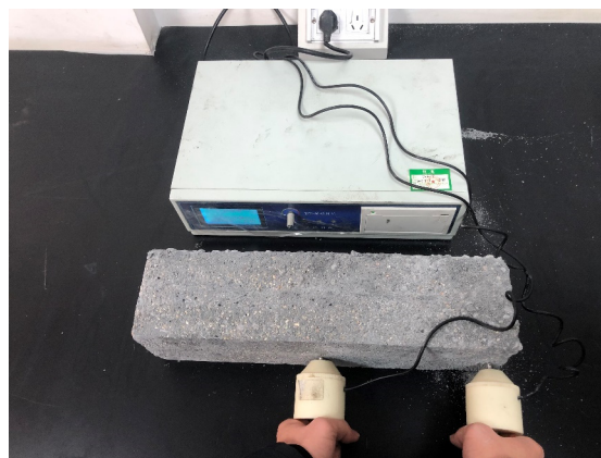
Figure 3. Equipment for measuring the RDEM of concrete specimen.
