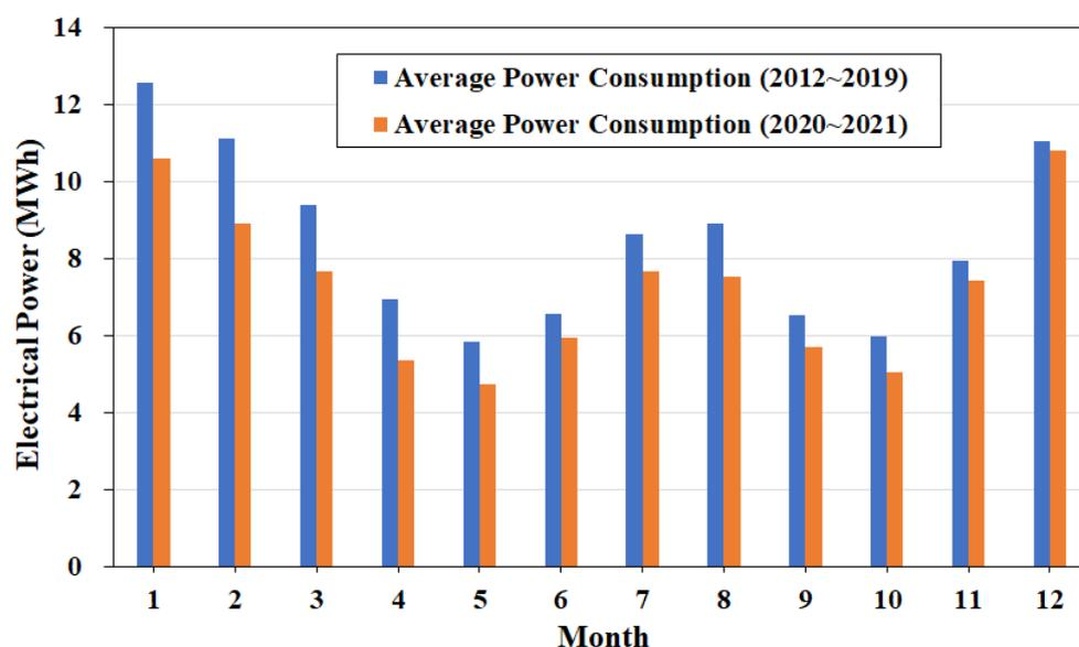
**Figure 5.** Monthly cumulative power consumptions during 2012–2019 (blue bar graph) and 2020–2021 (orange bar graph).
