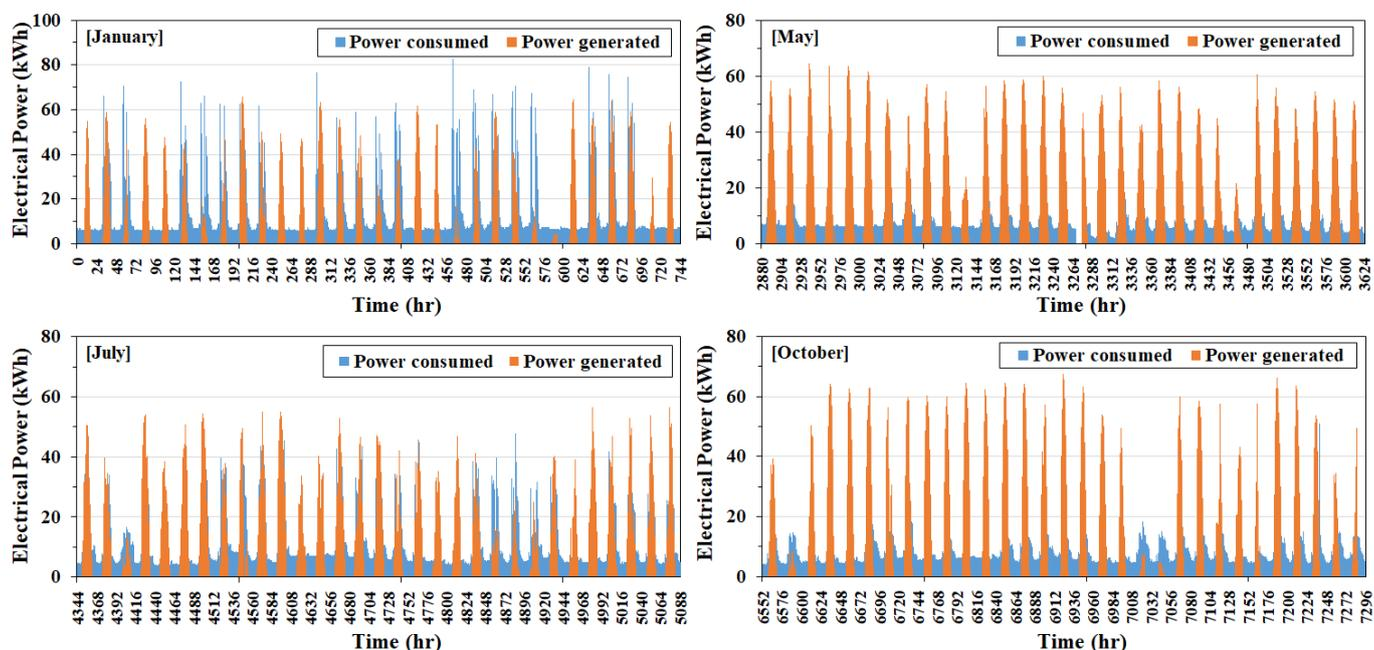
Figure 17. Variations in the real-time power generation and consumption in representative months.
