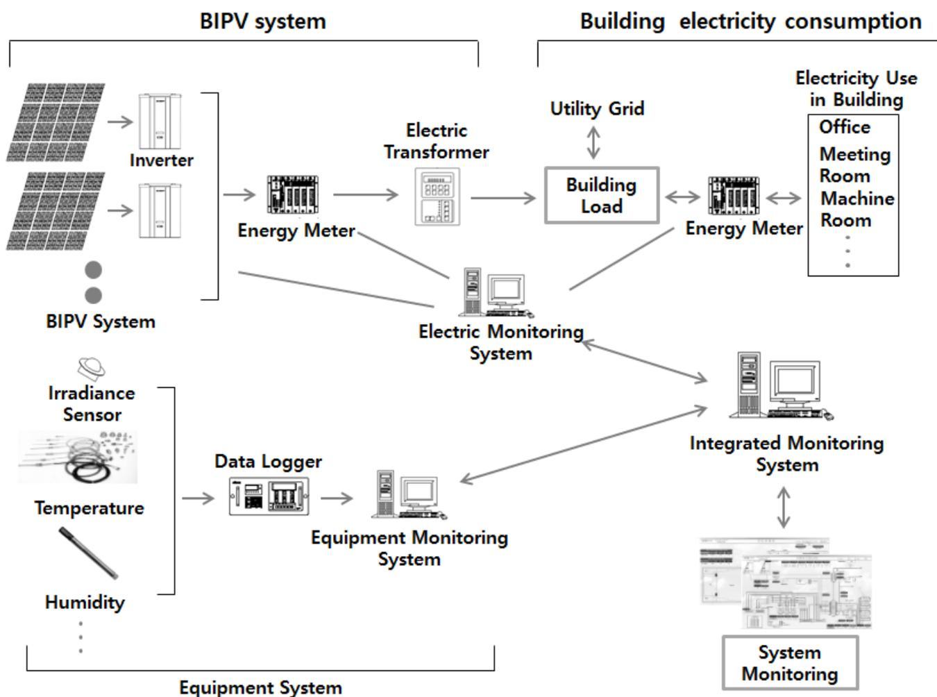
Figure 3. Schematic of the data monitoring and storage system.
