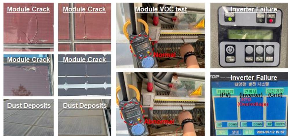
Figure 11. Major faults for photovoltaic (PV) system.
