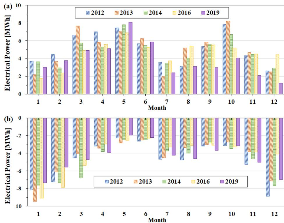
**Figure 14.** Differences in monthly cumulative (a) surplus power and (b) shortage power based on hourly data.
