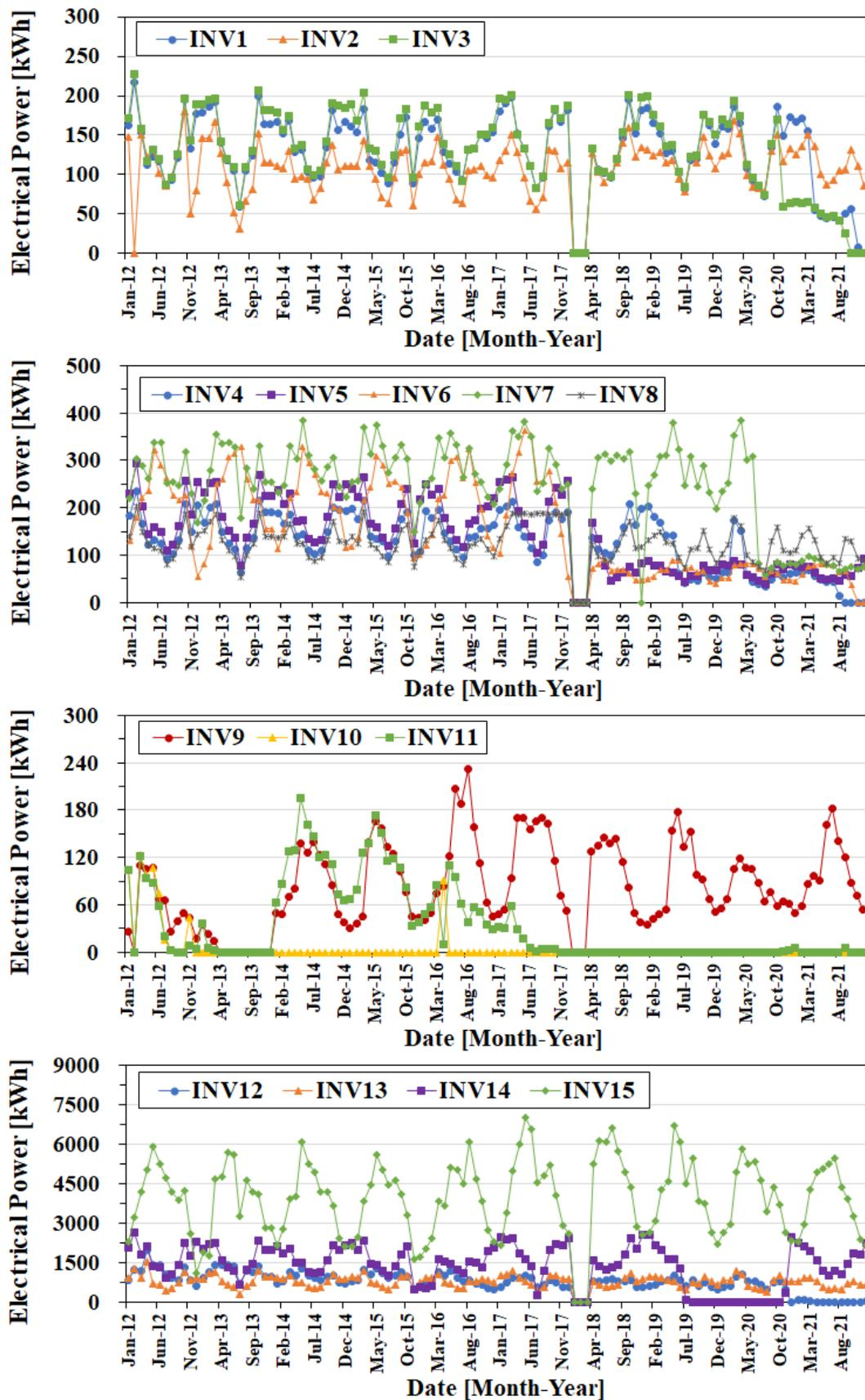
Figure 10. Monthly cumulative power generations of all of the inverters (INV1–INV15).
