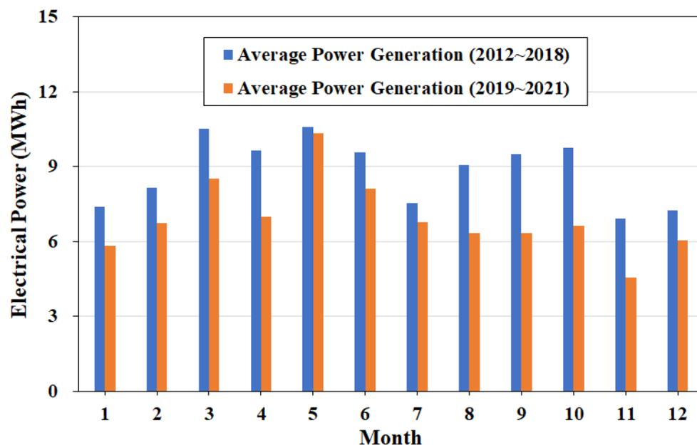
Figure 9. Monthly cumulative power generation during 2012–2018 (blue bar graph) and 2019–2021 (orange bar graph).
