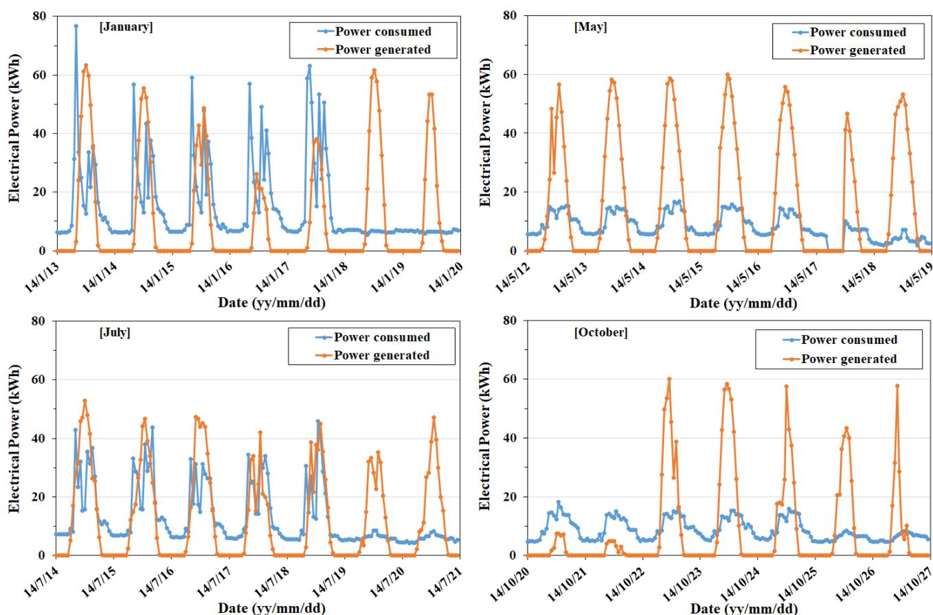
**Figure 18.** Variations in the real-time power generation and consumption for a week in representative months.
