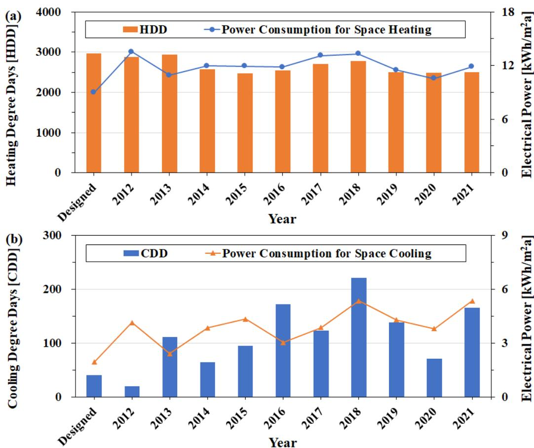
Figure 7. (a) Heating degree days and power consumption for space heating; (b) cooling degree days and power consumption for space cooling.
