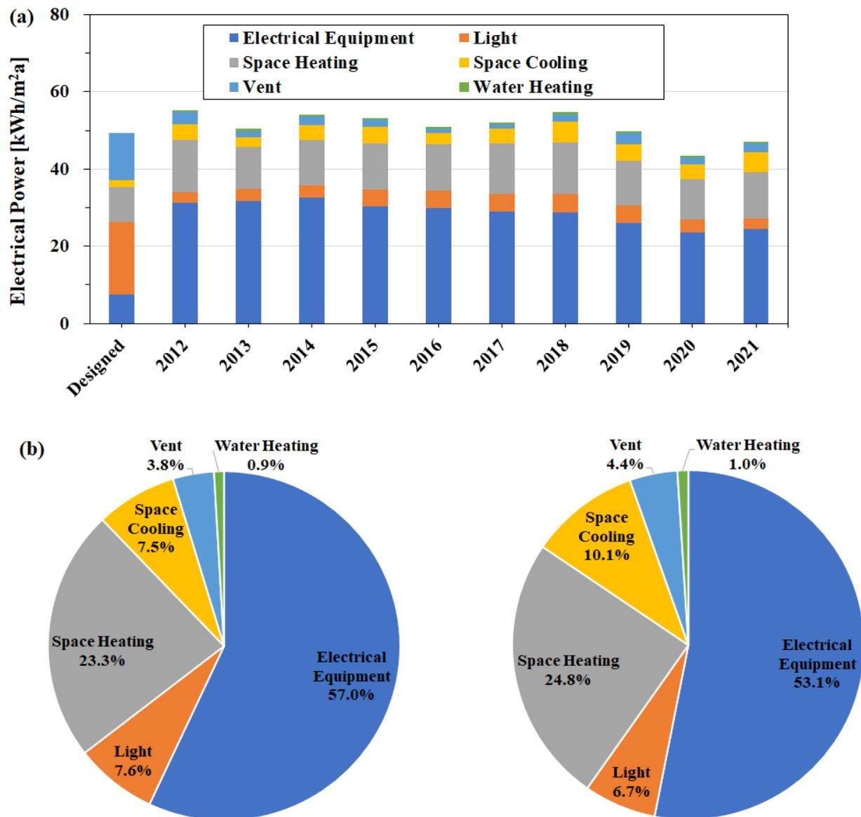
**Figure 6.** (a) Power consumption by end use during 2012–2021; (b) comparison on the proportions of power consumption by end use between different periods (2012–2019 and 2020–2021).
