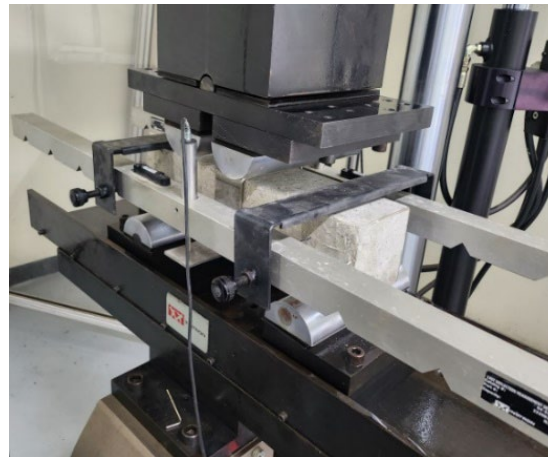
Figure 2. Test setup of flexural performance following ASTM C1609 [21].
