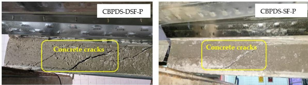
**Figure 11.** Typical concrete cracks failure inside the C-purlins beam.
