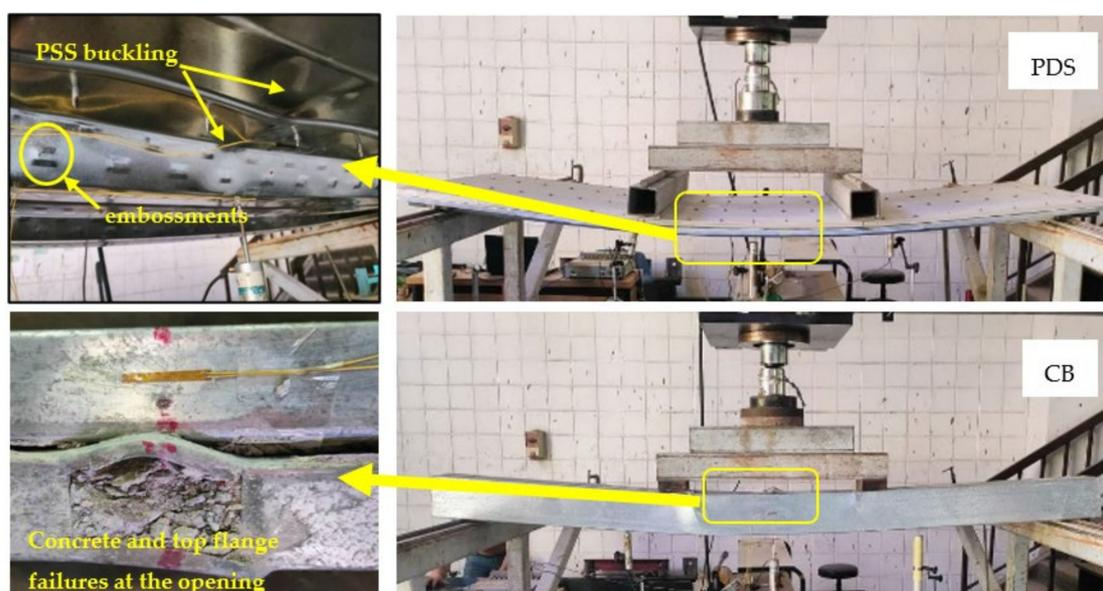
**Figure 9.** Typical bending behavior of control specimens PDS and CB.
