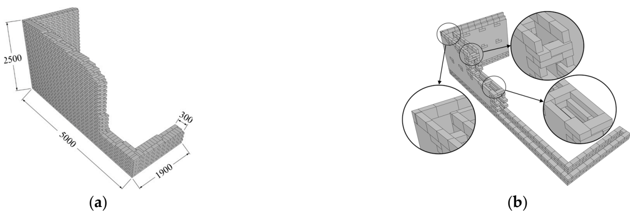
Figure 3. Stone unit layout for (a) double-leaf wall specimen (dimensions in mm) and (b) three-leaf wall specimen (the middle of the wall was filled with rubble).
