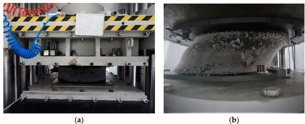
Figure 4. For -20\text{ }^{\circ}\text{C} , 24 h exposure time loading combination (a) LRB placed in the seismic isolator test device (b) a view from cyclic motion.
