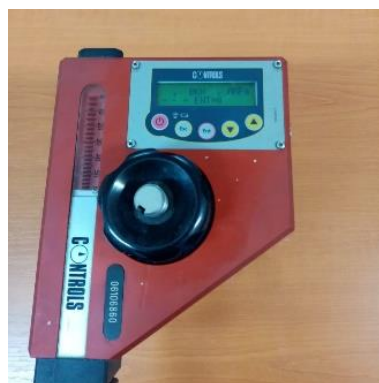
Figure 9. Apparatus for testing adhesion to the support layer.
