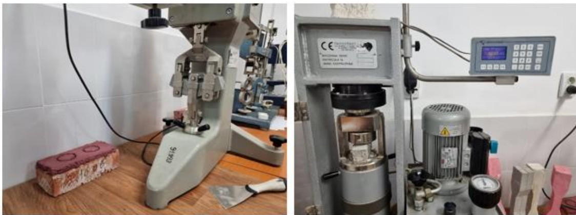
Figure 8. Determination of bending (left) and compressive (right) strength.
