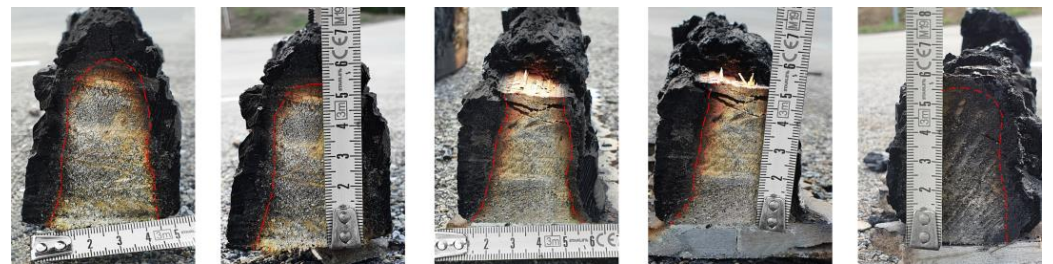
Figure 10. Residual cross-sectional areas of the timber elements after the test.
