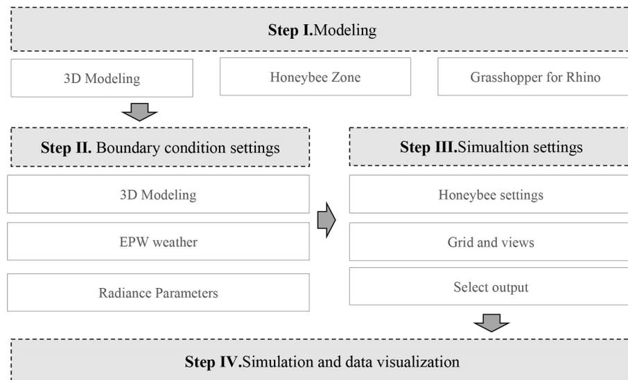
Figure 8. Daylighting simulation process.
