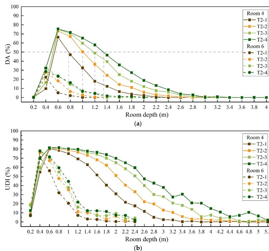
**Figure 12.** The effect of window width changes on room daylighting performance. (a) DA, (b) UDI.
