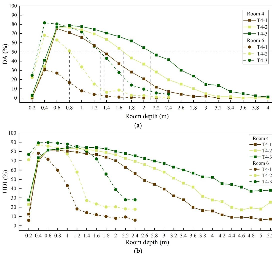
Figure 14. The effect of patio width changes on room daylighting performance. (a) DA, (b) UDI.
