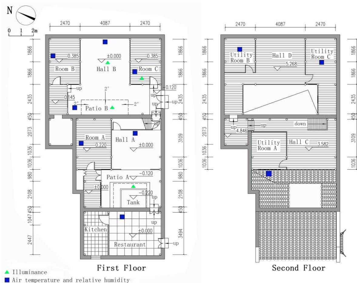
**Figure 4.** Plan view of test house showing the monitoring points.
