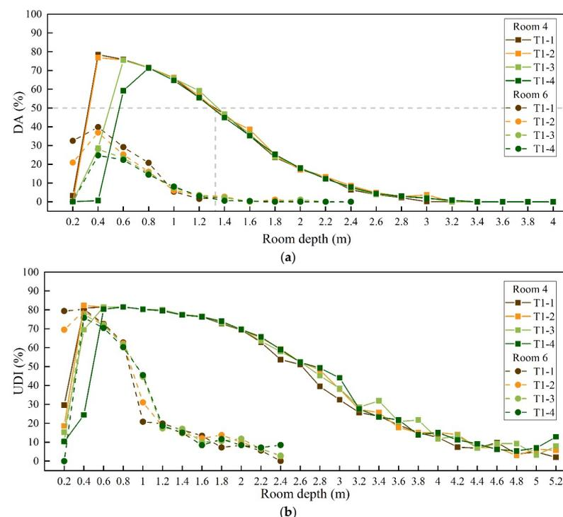
**Figure 11.** The effect of window edge height changes on room daylighting performance. (a) DA, (b) UDI.
