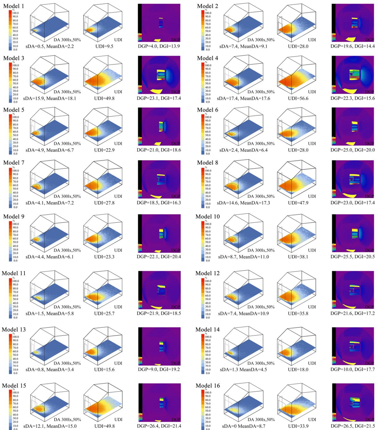
**Figure 10.** Simulation results of 16 orthogonal models.
