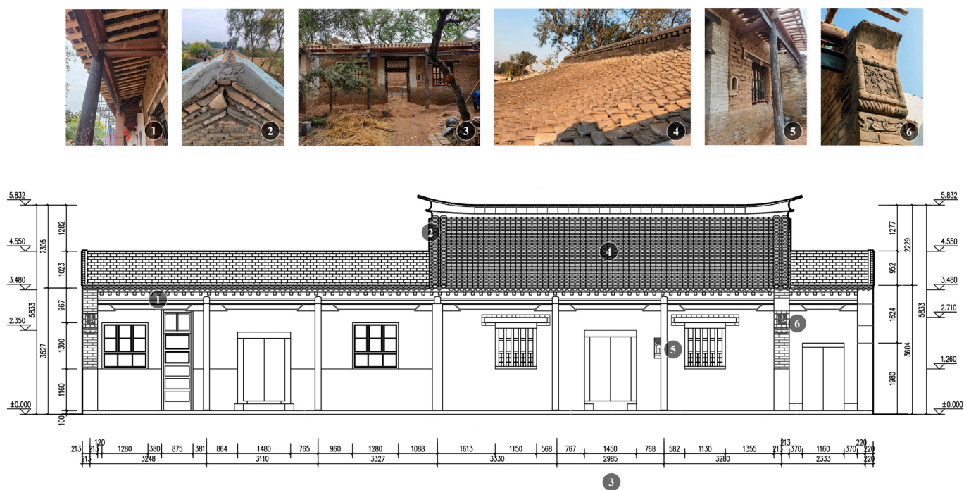
Figure 10. Building and courtyard façade and main components.
