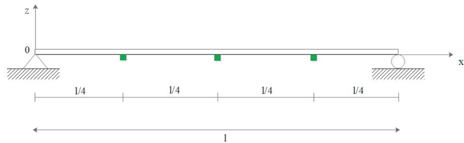
Figure 19. Simply supported beam and sensor locations.
