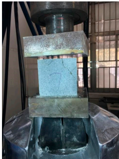
Figure 7. Schematic diagram of the uniaxial compression test.
